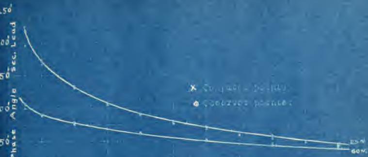
Fig. 5. Phase Angle Curves of Transformer.
